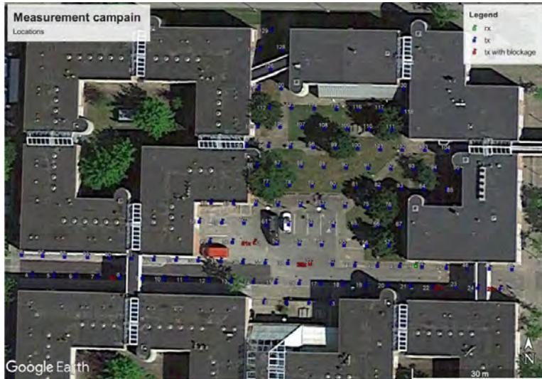
Figure 3.14: Anritsu's Courtyard Measurement Map and Locations of the Tx (130 locations) and the Rx
