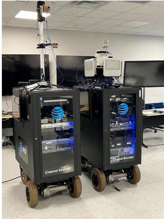
Figure 3.5: AT&T's Channel Sounder Setup for Indoor Communication Measurements
