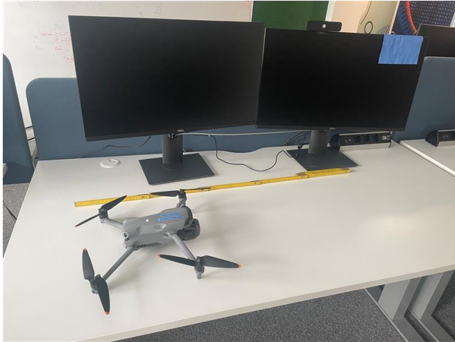
Drone: DJI Air3, 920g, C2 class, 259 × 326 × 106 mm (L×W×H)
